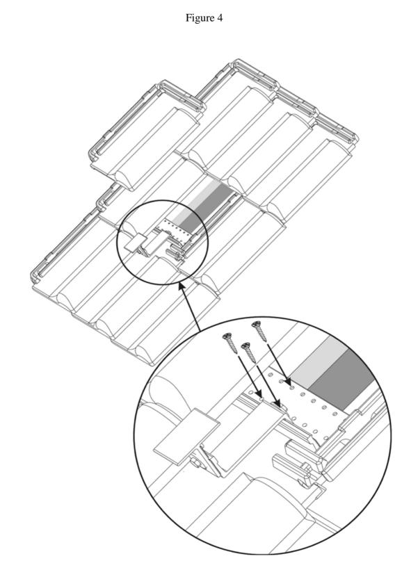
After verifying the proper attachment of the base, the tiles are placed in to their position and they retested for their excellent adaptation, not to leave loopholes that will allow water inflow.
