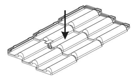
We continue with the installation and the rest support bases and after completing this task, we place the aluminum rails. The rails are placed horizontally or vertically in relation to the provision of tiled roofs, as shown in Figure 6 and 7.
