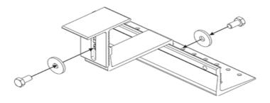
After assembling the base, the tightening to the rafters follows. The base is always placed perpendicular to the rafters and screwed in at least three (3) points, as shown in Figure 4.
