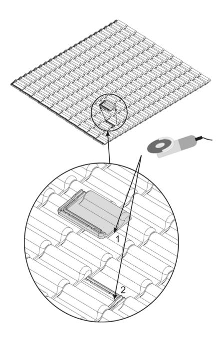
The second step is to assemble the Tile Roof Base, as shown in Figure 3. The Base packing box includes all the necessary materials.
